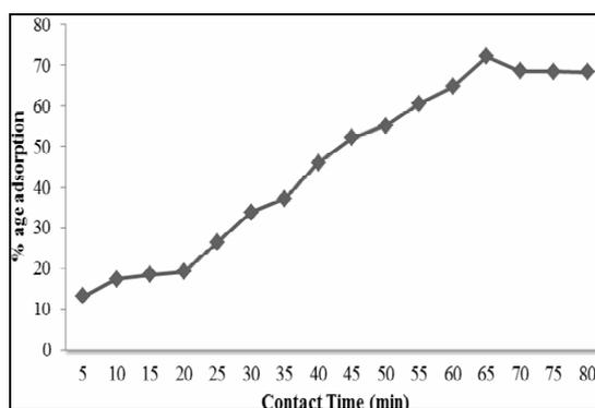
Fig. 5: Effect of contact time between Acid Yellow-73 and C.R.P on % age adsorptive removal of dye.
