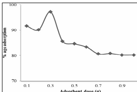
Fig. 7: Adsorbent dose effect on % age adsorptive removal of Acid Yellow-73 dye by chemically modified C.R.P.
