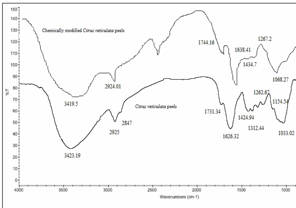
Fig. 3: FT-IR spectrum of unmodified and chemically modified *Citrus reticulata* peels.
