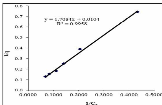
Fig. 9: Langmuir graph for adsorptive removal of Acid Yellow-73 dye by chemically modified C.R.P.
