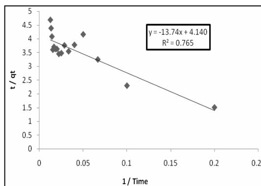
Fig. 12: Pseudo-second order graph for adsorptive removal of Acid Yellow-73 dye by chemically modified C.R.P.
