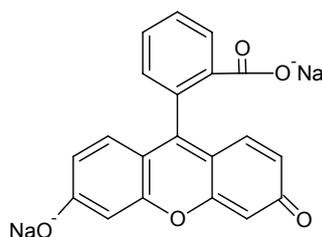
Fig.1: Chemical structure of Acid Yellow-73 dye.
