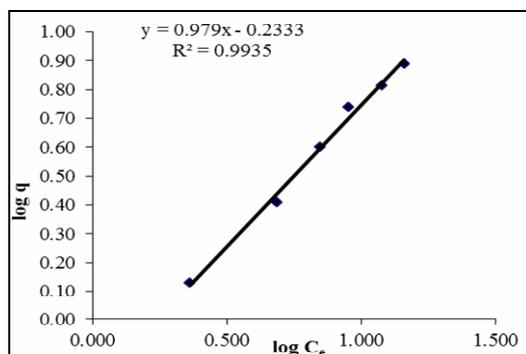
Fig. 10: Freundlich graph for adsorptive removal of Acid Yellow-73 dye by chemically modified C.R.P.
