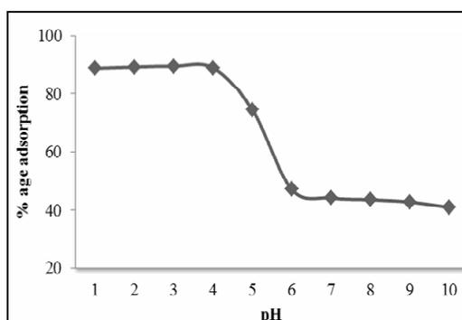
Fig. 4: Solution pH effect on % age adsorption of Acid Yellow-73 dye by chemically modified C.R.P.
