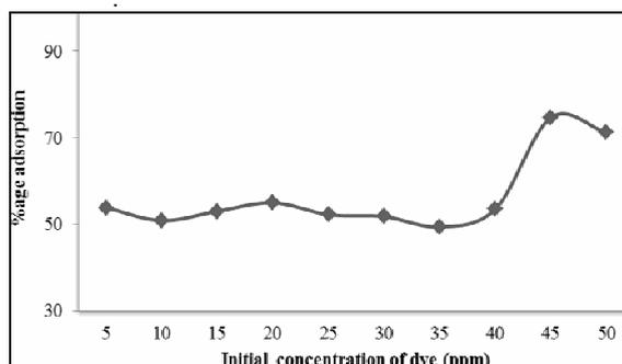
Fig. 8: Initial concentration of dye effect on % age adsorptive removal of Acid Yellow-73 dye by chemically modified C.R.P.
